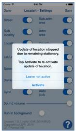
Update of location is terminated and Auto-lock is turned on (activated) – all of it is done to save device battery.
